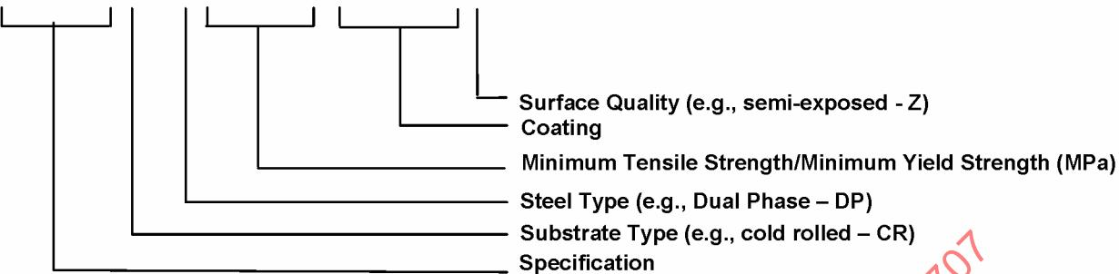
Advanced high strength cold-rolled hot-dip galvanized dual phase steel per SAE J2745 CR DP490T/290Y HD70G70GZ. Cold-reduced hot-dip galvanized dual phase steel with min. tensile strength of 490 MPa and min. yield strength of 290 MPa, for a semi-exposed application.
