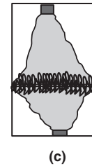
View from (b) of unwanted spray collision and creation of voids if the spray pattern in (b) is not used
