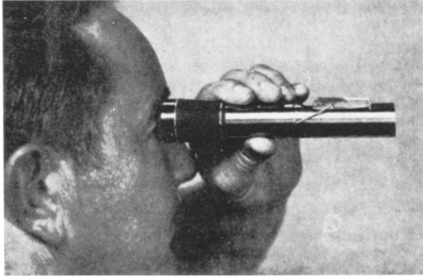
Figure A-4-2.2(b) Holding this type of refractometer up to a light source to take a reading where the dark field intersects the numbered scale.
