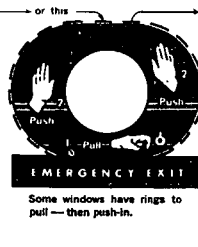
Figure A-1. The principal points to consider in gaining access to civil transport aircraft. Each aircraft must be examined individually to know how doors and windows may be most easily opened from outside.
