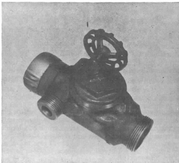
A combination check and bleeder valve used at the pumper when vertical lift is 200 ft (61 m) or more. A check valve holds the water back when a positive displacement pumper is stopped.
