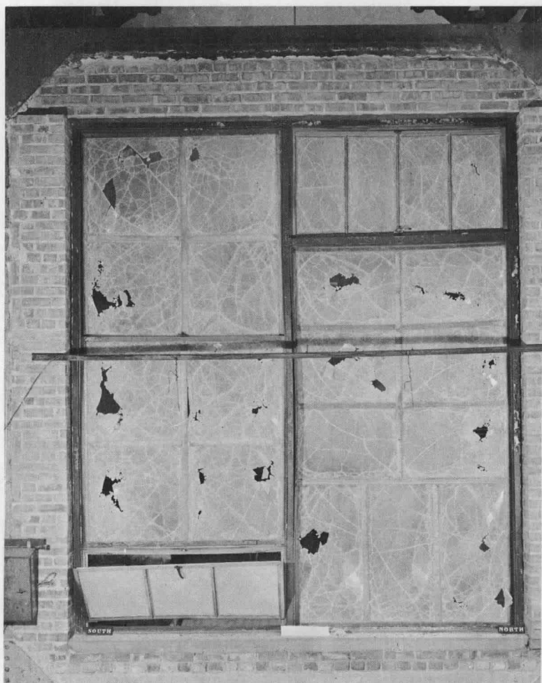
Unexposed side of window assembly after fire exposure and hose stream application.
