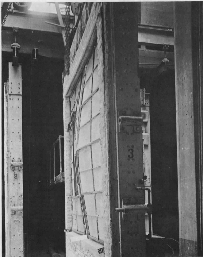
Exposed side of window assembly after fire exposure and hose stream application.
