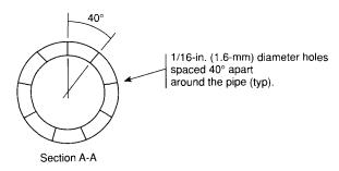
Figure 4-2.1(b) Pressure probe.
