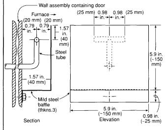
Figure 4-2.1(a) Static pressure-measuring device dimensions.
