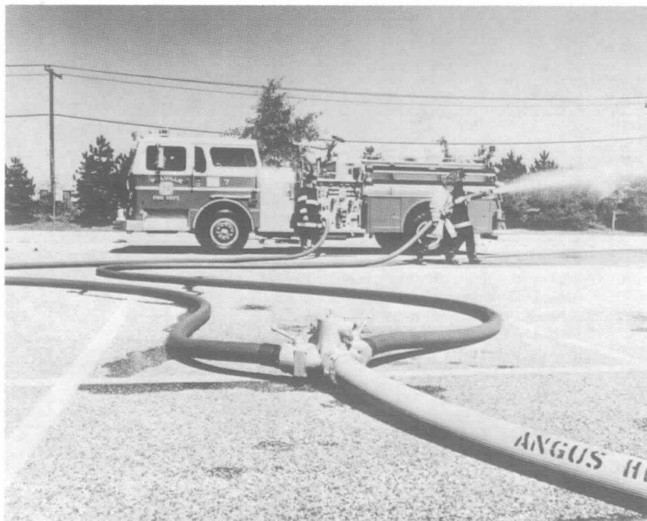
Figure D-1-7. Large diameter hose supplying a distribution valve from which run two 2½-in. (65-mm) lines, one to a hand line and the other to supply a pumper.
