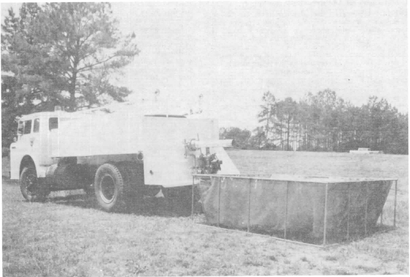
Figure C-1-13. A mobile water supply (tanker) mounted on a truck chassis of the 27,500 GVW range. Capacity of tank is 1250 gal (4731 L) and can be filled from draft in approximately 4 minutes and discharged in approximately 95 seconds.
