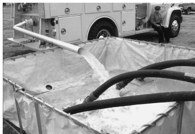
FIGURE C.15 Portable Drop Tank with "L"-Shaped Aluminum Irrigation Discharge Pipe.
