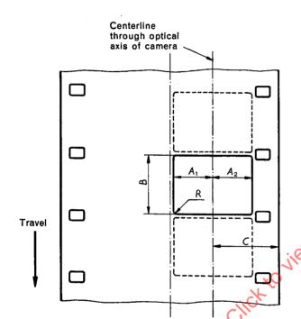
The camera aperture plate and the camera film registration device should be so related dimensionally that the framelines between the images are coincident with the centerlines of the sprocket holes.
