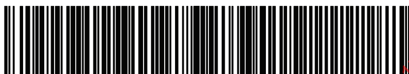
Figure B.3 — Code 128 encoding “25SUN043325711MH8031200000000001”
