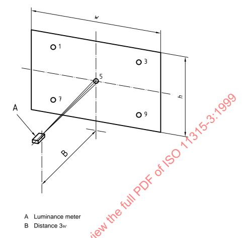
Figure 5 — Arrangement for determining the uniformity of luminance
