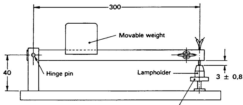
Support to raise lampholder so lever arm is in horizontal position when force is first applied
